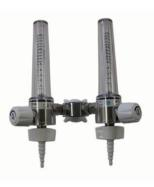
The  $\text{RTM}_3$  flowmeter is also available in a twin setup model. This allows the user to run two flowmeters off the one gas outlet. This is set in "Y" configuration, with each flowmeter operating independently of each other. The standard setup is for oxygen, but it is available for other gases (ie. Air, Carbon Dioxide, Carbogen) upon request.
